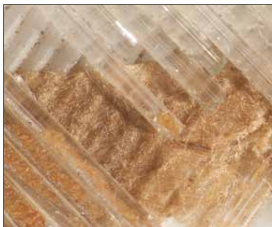
Fig. 6: Photomicrograph of an edge of panel 2010.6.26 showing the hollow area in the center of the glass rods and the layering of paper and rods.
